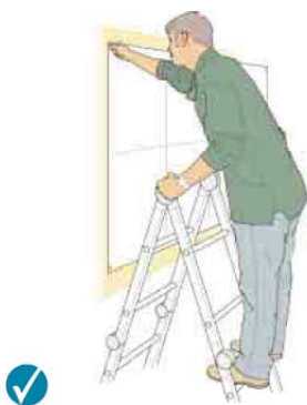
Figure 6a Correct – two clear rungs. Don't work any higher up this type of stepladder.
