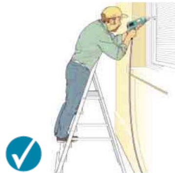
Figure 7b Correct - steps facing work activity
