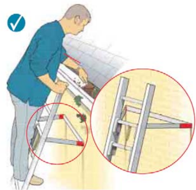
Figure 2 Stand-off device and working maximum height on a ladder
