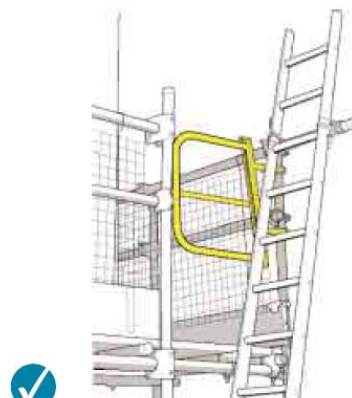
Figure 4 Access ladders tied and extending above the landing point
