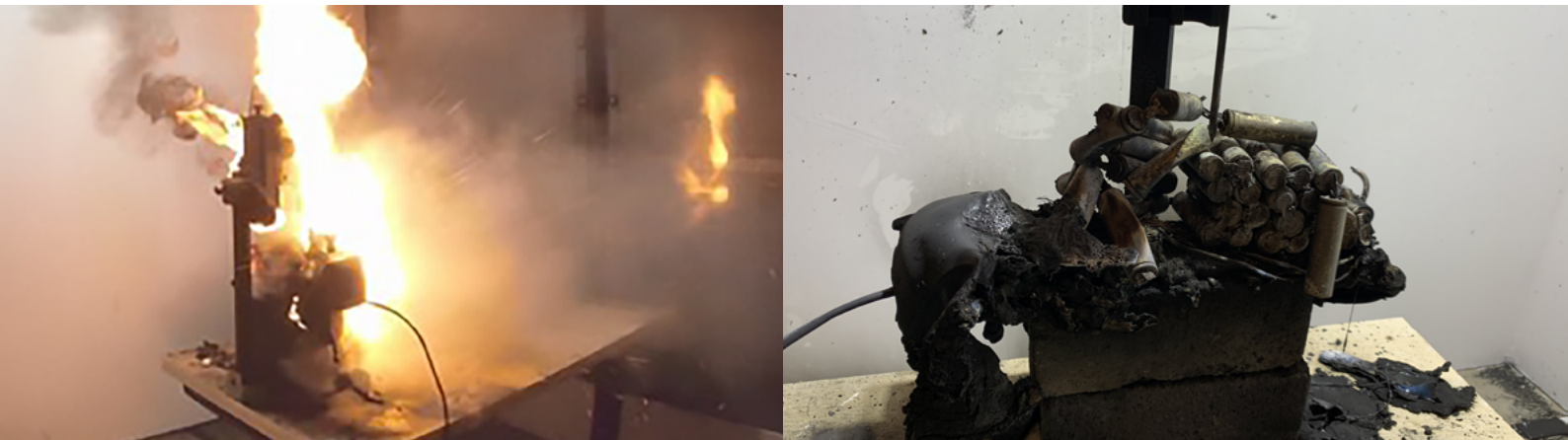
Figure 29: Photos of test sample during and post thermal runaway event from a simulated nail penetration test.
