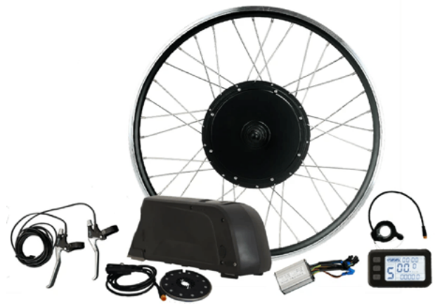
Figure 12: A typical conversion kit.
